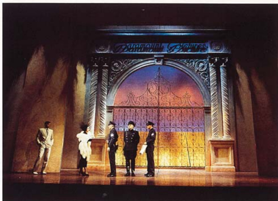
The Paramount Studio gate, formed from flying panels capable of travelling at two metres per second. Note the shadow projections.
