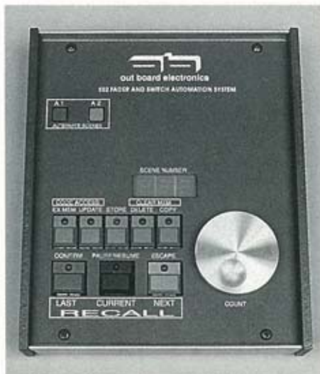
Outboard Electronics' automation system as attached to the Soundcraft Europa.
