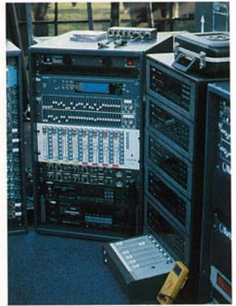
One of the processor racks with BSS compressors, BSS and Drawmer noise gates and Orban parasound parametric EQs.
