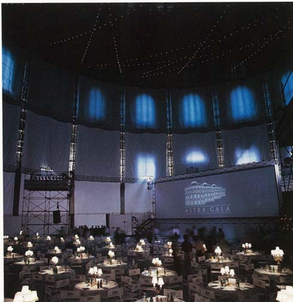
Venue: a municipal gasometer, Vienna. The disused circular building was used by Opel for a presentation. Trussing was TAS and scaffolding Kwik Form. 20 Verlinde motors and 15 Felco hand chain blocks were employed. Rigging consultant was Eddie Campbell of Arrow Rigging.
