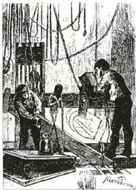
Lime-light men operating in the fly gallery. An illustration from 'The Graphic' in January 1874, reproduced from 'Theatre Lighting in the Age of Gas' by Terence Rees.
