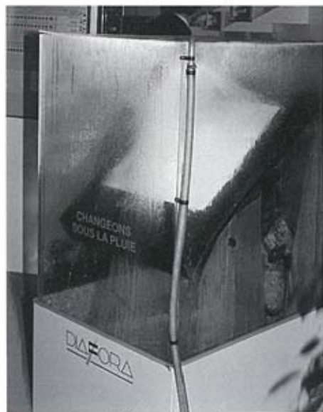
Soak test for a Diafora colour changer.
