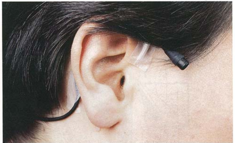
Over-the-Ear radiomic showing clip and cable taped in position.
