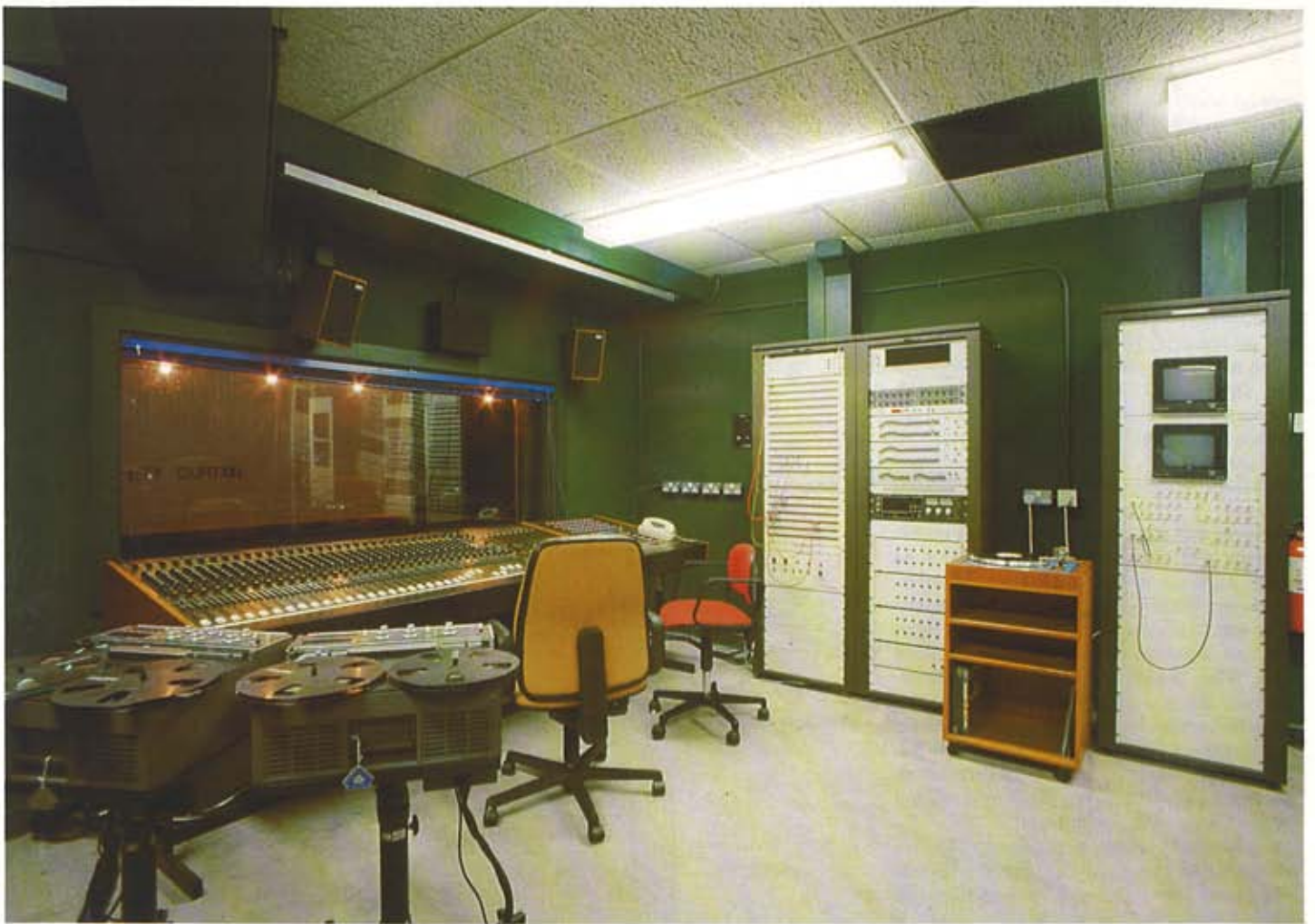
Lyric Theatre Sound Control—32 into 8 PEP Mixer & Revox tape decks.
