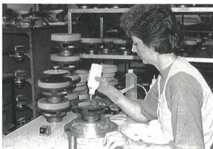
Operator Ann Linsey applies adhesive to loudspeaker chassis prior to inserting and centralising the HF voice coil assembly.
