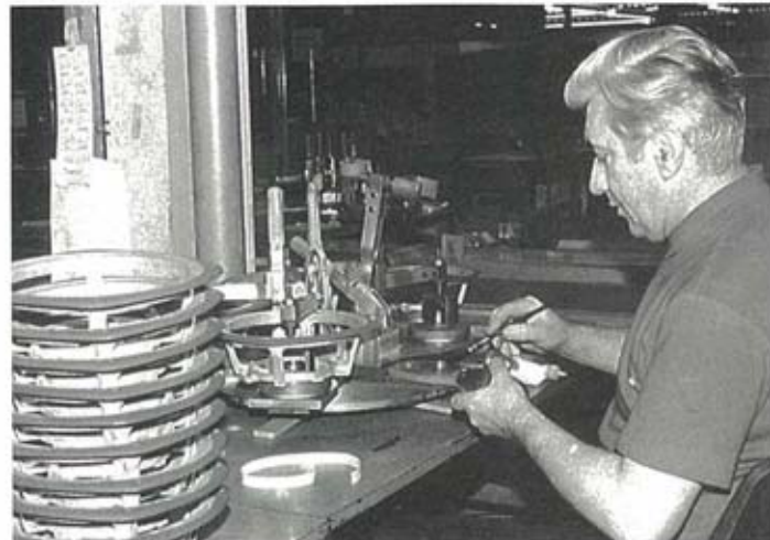
Operator Bill Watson carefully assembles magnet to frame parts.
