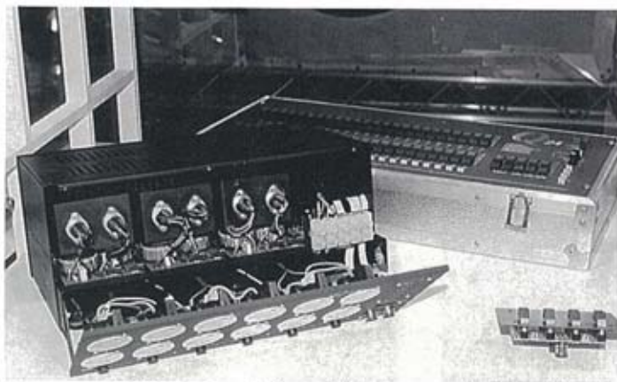
Easy access to Lightfactor's new 6 channel digital powerpack with Q24 board in background.
