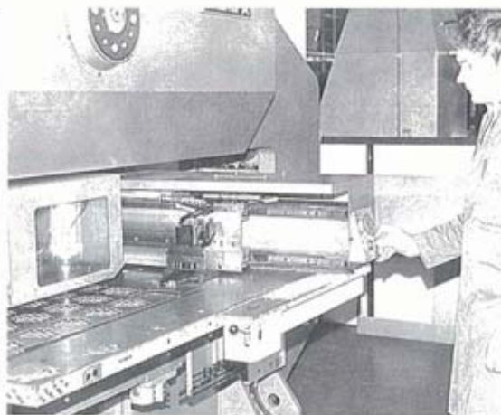
The Amada CNC Pega 40-ton 58 turret punching machine making wireguards for the Quartet with the finished product (above) at approximately 1/3 size.
