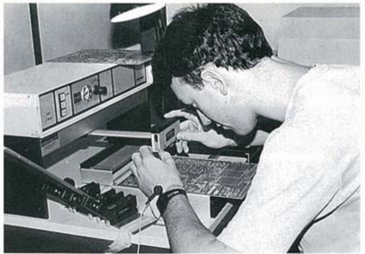
Surface mount placement for the ASIC's used in EC90 dimmers.
