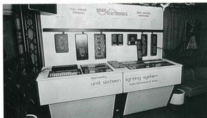
Mode's display included their wall-mounting 16 channel digital pack, available in both dimming and non-dimming versions.
