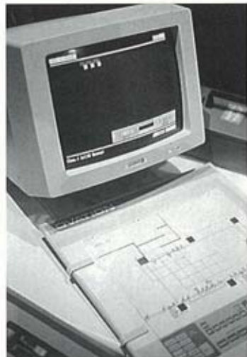
Eurolight's Ovation control system with graphic tablet.
