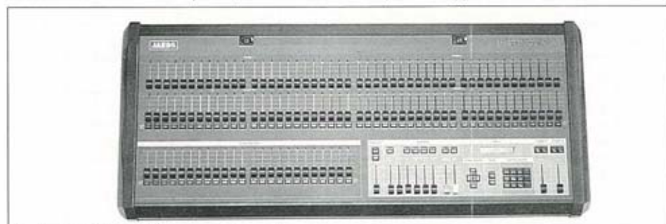
The Jands Instinct lighting control console.
