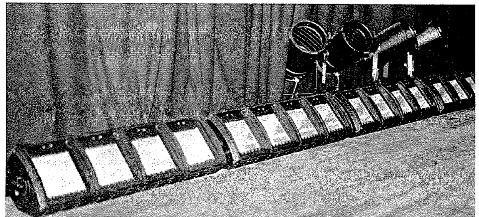
5 groups of 4 Strand Coda battens (500W) are located against the back wall (a further five groups act as the floor bar). Also in picture is a group of four Strand Punchlites.
