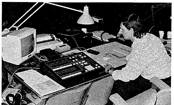
Krystof Kozlowski at work with his 'mouse' on the ADB S20 lighting control system.
