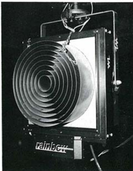
A Rainbow followspot scroller in use on a R&V 1k low voltage spot.
