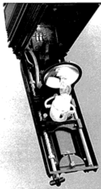
The Teatro Tratto 'G' range of zoom profiles, fresnels and PCs uses a G22 lamp base for either the 1000 watt T30, the 1000 watt CP71 or the new 1200 watt CP93 without the need to change the height of the lampholder. Shown here is the Tratto G fresnel with the G22 lampholder and focusing system in detail.
