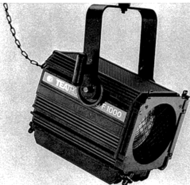
The Teatro Tratto 'G' range of zoom profiles, fresnels and PCs uses a G22 lamp base for either the 1000 watt T30, the 1000 watt CP71 or the new 1200 watt CP93 without the need to change the height of the lampholder. Shown here is the Tratto G fresnel with the G22 lampholder and focusing system in detail.
