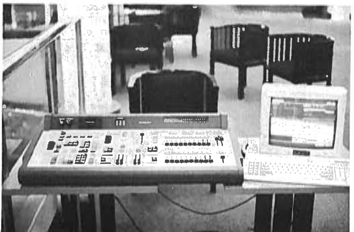
The Microlite Three memory lighting board - a new approach to lighting control, using 16 bit computer technology.
