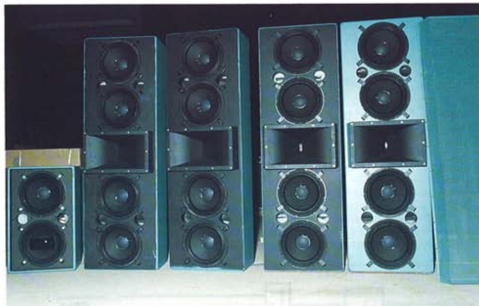
CX3 co-axial delay loudspeaker and CL1000 columns, midway through painting.
