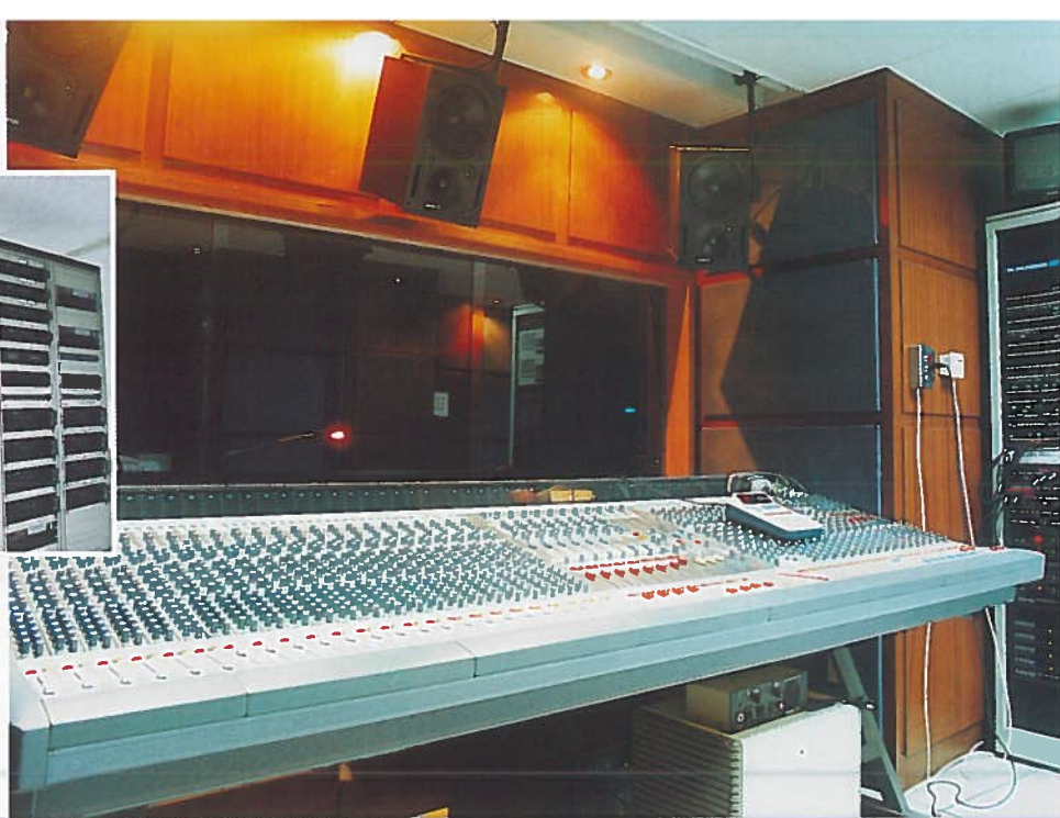
Right, the main Soundcraft Europa mixing desk in the control room. Inset, the amp rack
