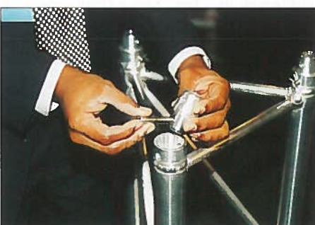
Tomcat's John James demonstrates the company's new in-line truss connector.
