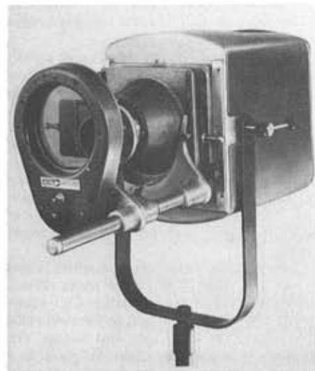
The original CCT Halostar with polaroid spinner - used for moving effects.
