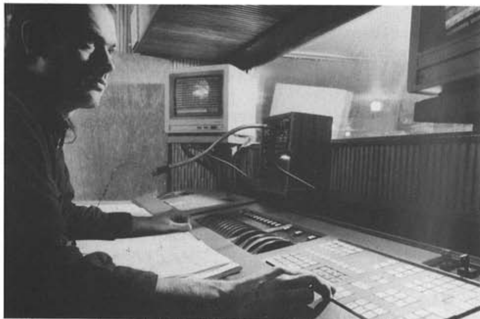
The Siemens computer controlled Sitralux B40 lighting control system at the Royal Opera House.
