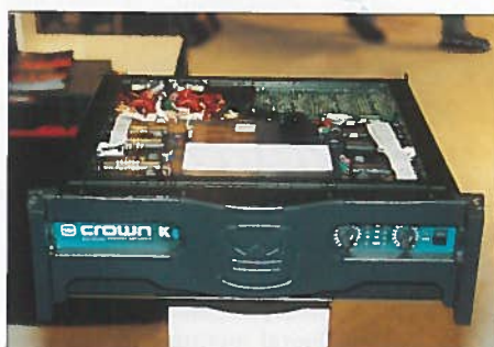
The new K4 amplifier from Crown - 5500W into 4 ohms bridged.
