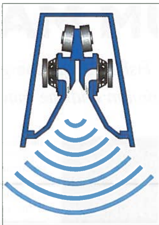
R-H's diagram showing the combination of mid and LF drivers in CoEntrant Waveguide Technology design.
