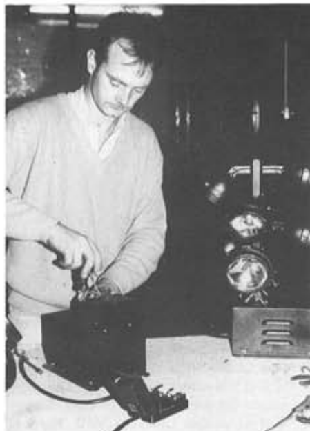
Assembly of the new SIS 'Octolite', an 8-head Par 36 spinner. By staggering the positioning of the lamps, the beams from the Octolite will fill almost any shaped room. The pods can all be pointed in a multitude of directions.
