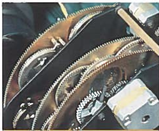
Effect and gobo wheels for superimposing rotating gobos, prisms, and effects
