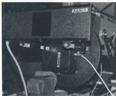
A Pani BP1.2 1200w HMI projector fitted with effects wheel, effects lens, and electronic dimming shutter pictured at AC Lighting of High Wycombe.
